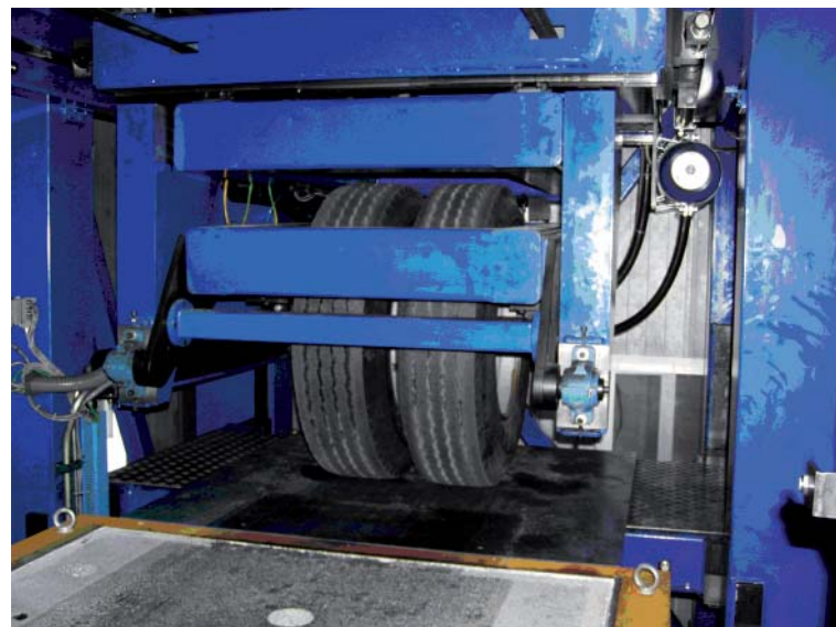
DART, with dual wheel mounting, in the off-loaded state. The pavement test slab is visible in the front of the picture.
